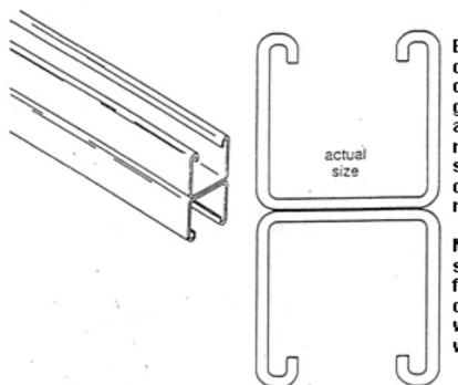
Back to back and combination channels provide greater flexibility and strength that may be needed in some areas of construction and maintenance.
